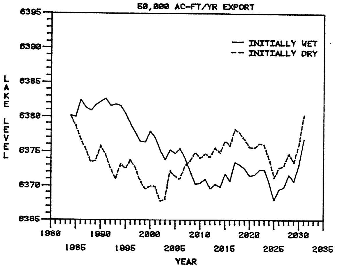
Figure 3-5c Comparison of Lake Level Fluctuations, 1985-2031, Using 1937-83 Hydroclimatic Conditions With Initial Sequence Above Normal (1937-46) and Initial Sequence Below Normal (1947-64)
