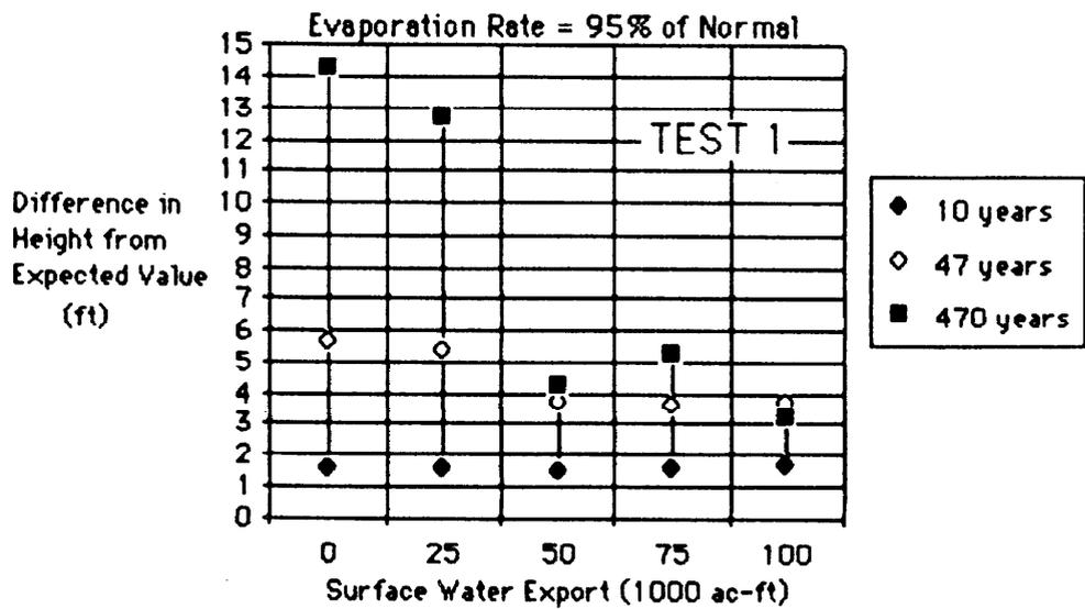
**Figure 3-13.** Sensitivity of Forecasted Lake Levels to Different Component Values
