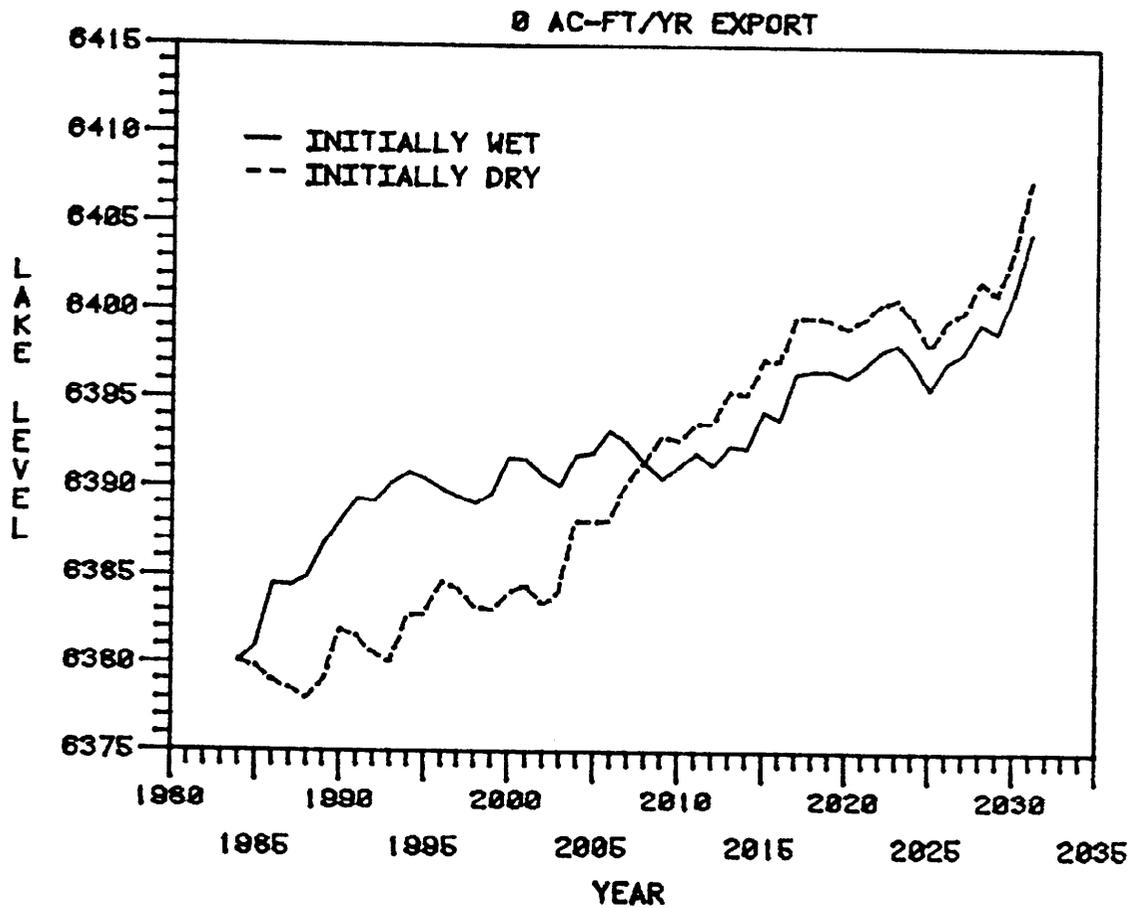
Figure 3-5a Comparison of Lake Level Fluctuations, 1985-2031, Using 1937-83 Hydroclimatic Conditions With Initial Sequence Above Normal (1937-46) and Initial Sequence Below Normal (1947-64)
