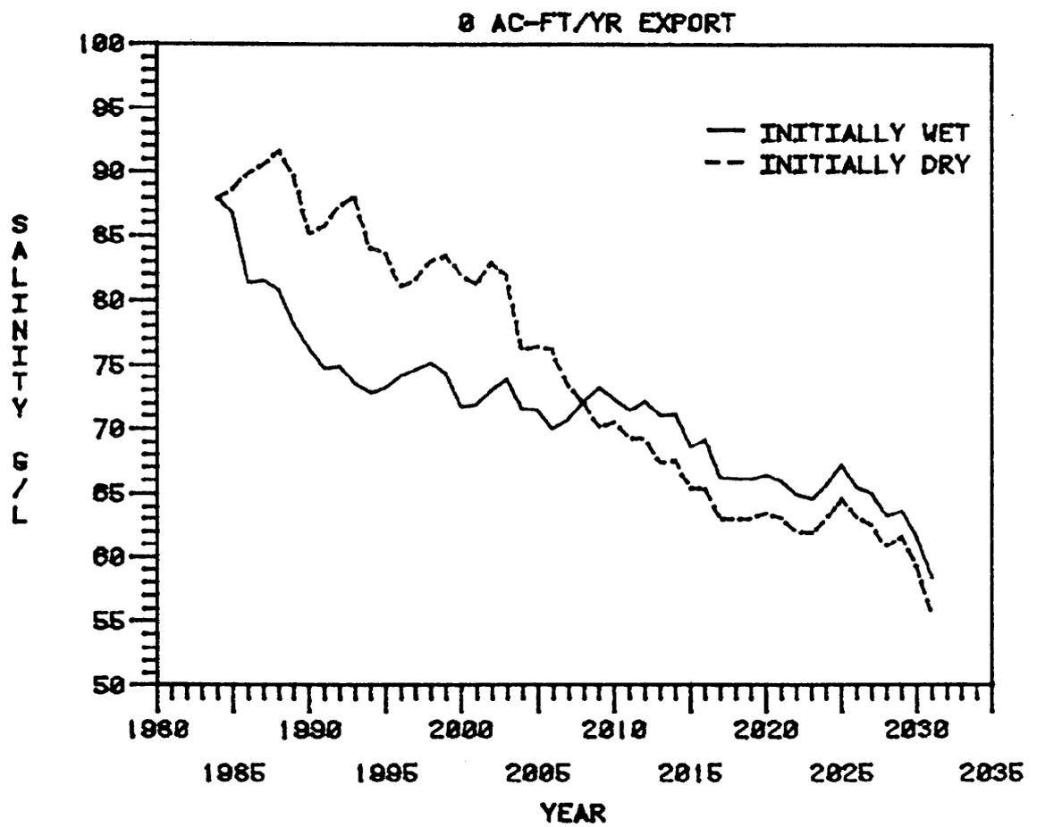
Figure 3-11a Projected Salinity Fluctuations Using 1937-83 Hydroclimatic Conditions With Initial Wet Sequence (1937-46) and Initial Dry Sequence (1947-64)
