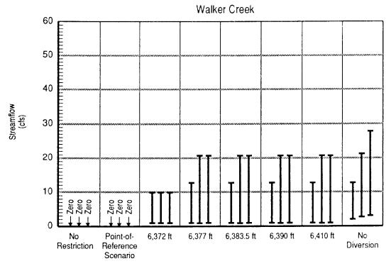
Note: The three bars for each alternative represent dry (20% driest years), normal, and wet (20% wettest years) conditions. The bars depict the annual range of monthly average streamflow. Runoff peaks occur in June or July, with the lowest flows persisting from September through March.
