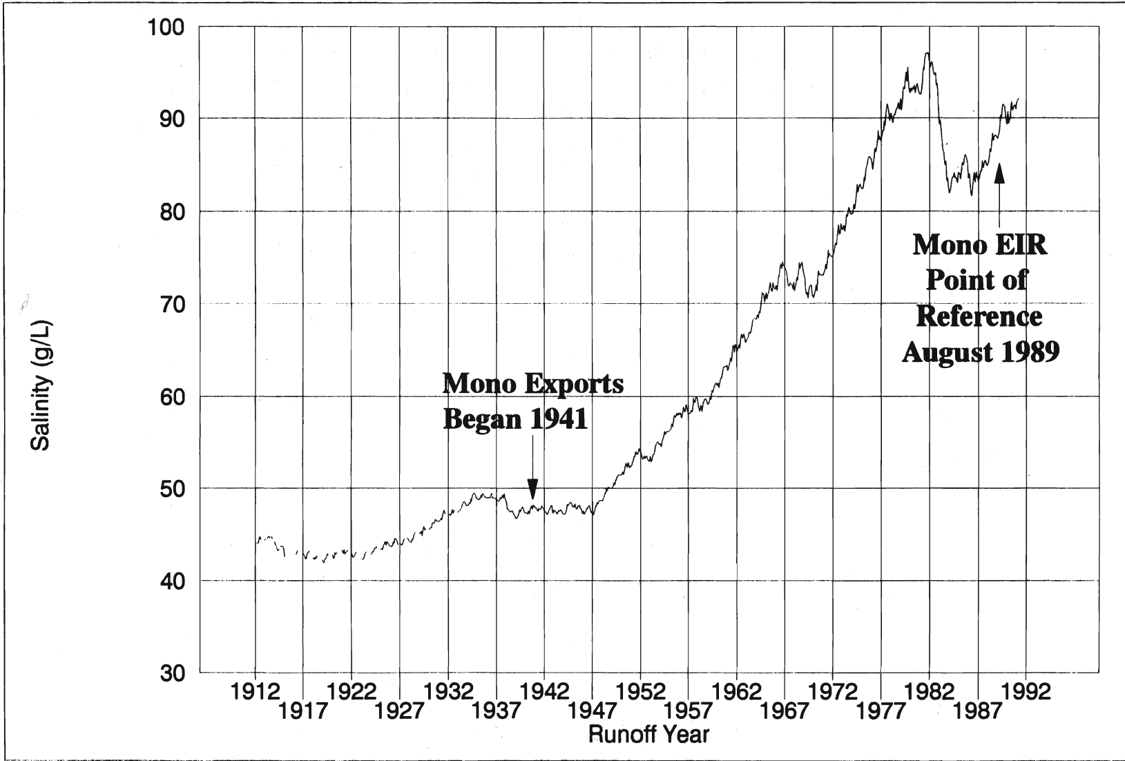
Figure 5. Calculated Mono Lake Salinity 1913-1991. (Based on Calculated Lake Volume and an Assumed Salt Content of 285 Million Tons)
