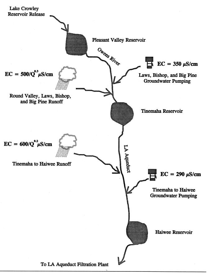
Figure K-5. LA Aqueduct Module
