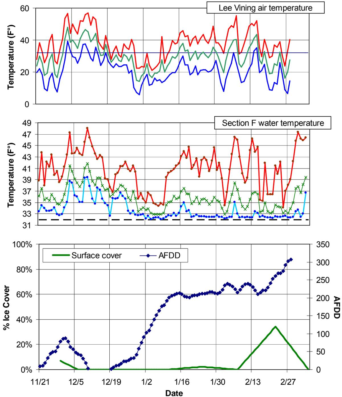
**Figure 16.** Tran\_FR percent ice cover (surface vs. subsurface cover), air temperature, water temperature, and AFDD (accumulated freezing degree day) between November 29 and March 7. Daily mean, maximum and minimum temperatures are shown as green, red and blue lines, respectively, for air and water temperatures. The air temperature data were obtained from Lee Vining. Water temperature was recorded in B1 Channel between Tran\_FR and Tran\_FP.
