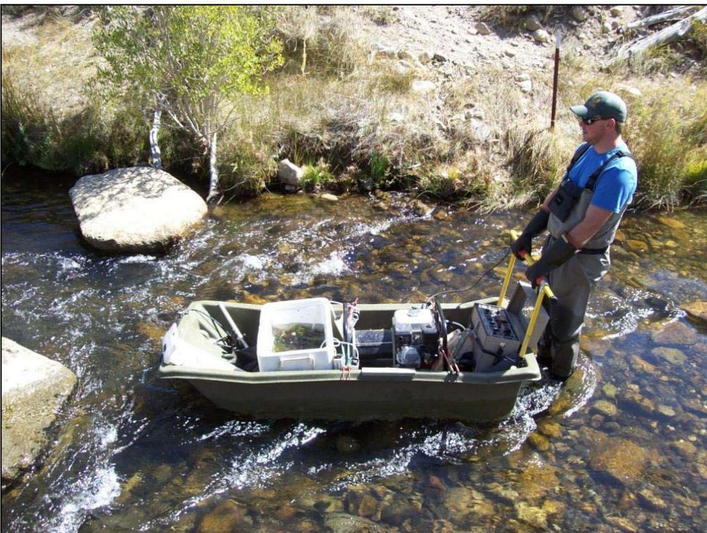
**Figure 5.** Electro-fishing barge with generator and cooler on Upper Rush Creek, 2009.
