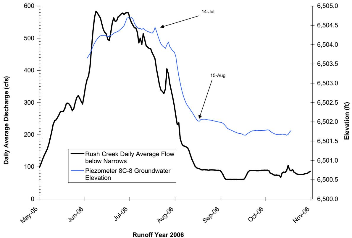
Figure 8. Rush Creek annual hydrograph and piezometer 8C-8 groundwater elevation for RY 2006-07.
