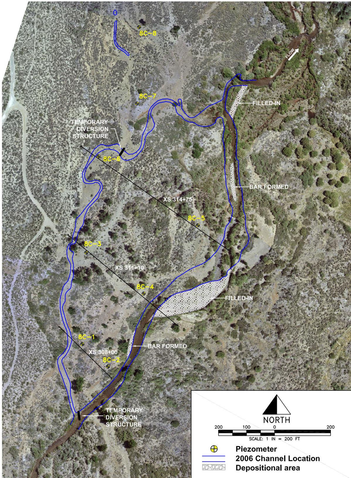
Figure 6. Location of piezometers and staff plates across the 8 Floodplain and field sketch map of channel realignment along the mainstem Rush Creek resulting from the RY 2006-07 snowmelt release.
