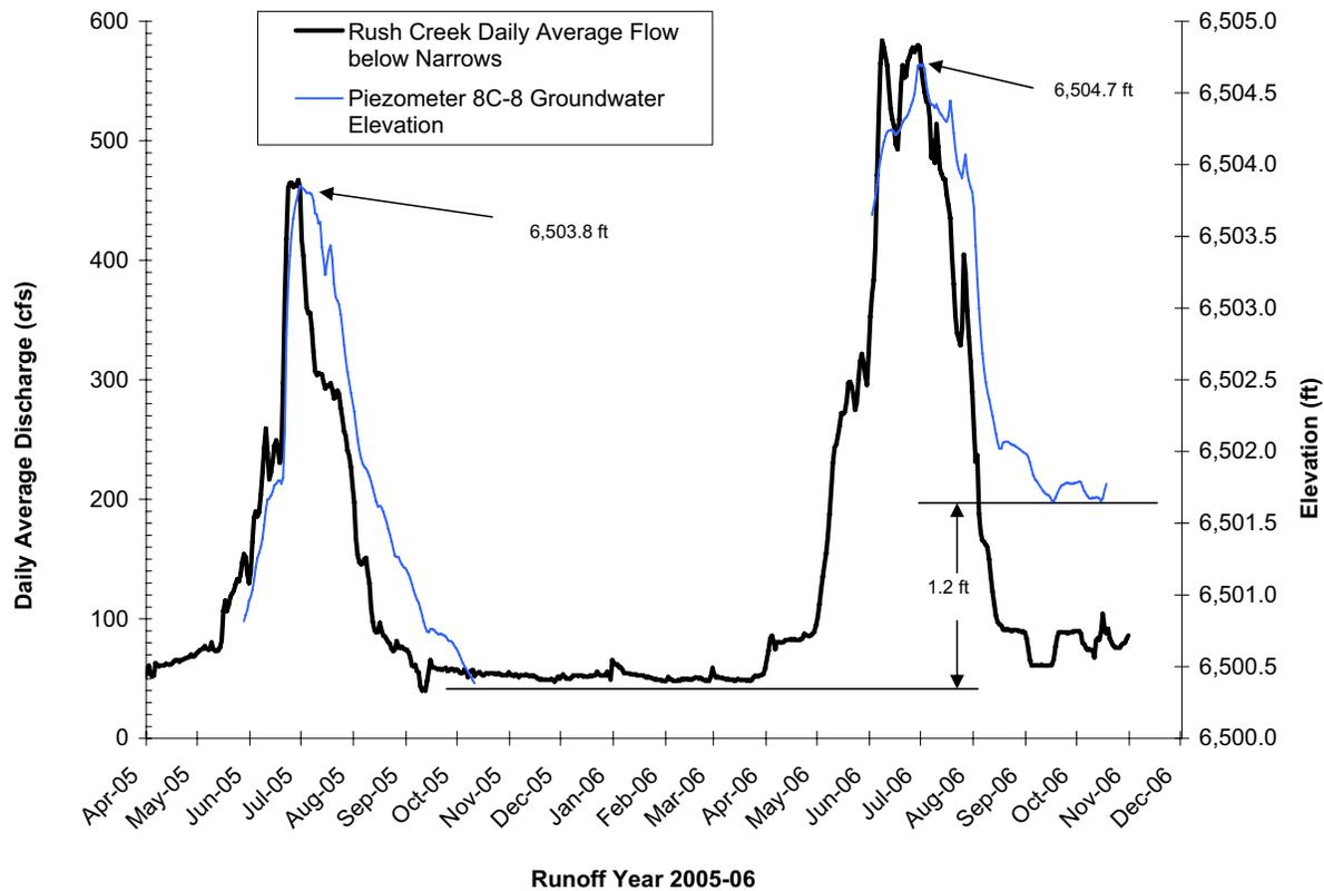
Figure 7. Annual hydrograph of daily average flow for Rush Creek below the Narrows for RY 2005 and 2006, plotted with groundwater elevation from the datalogger installed in Piezometer 8C-8.
