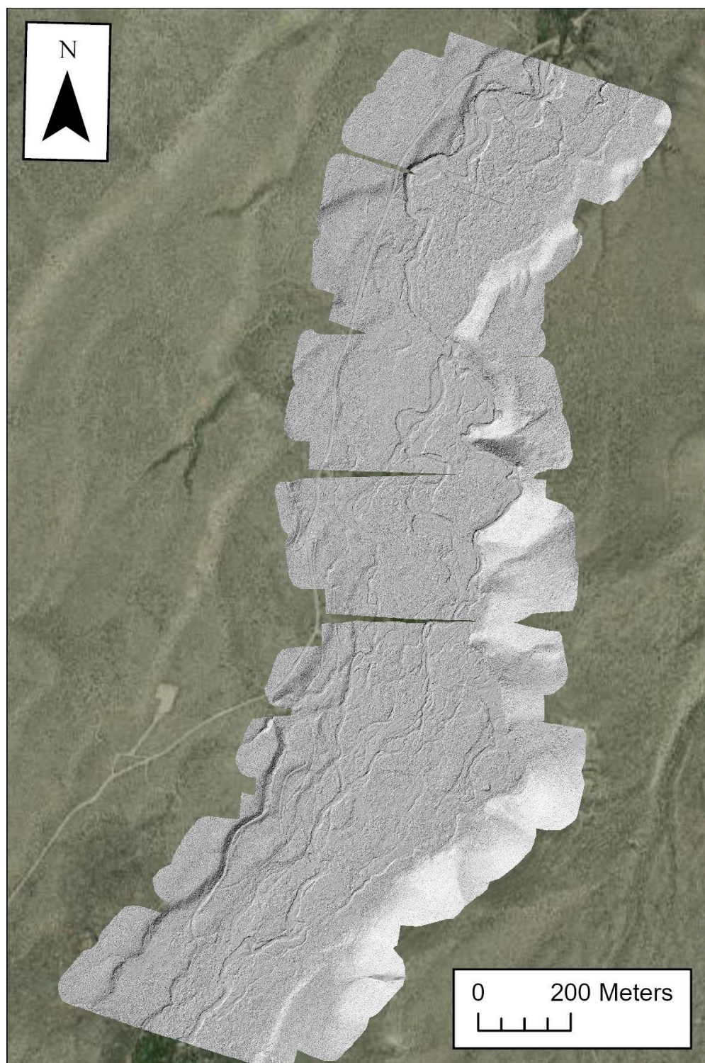
Figure 14. Hillshade of the 6" elevation dataset that was created from the 2024 LiDAR point cloud. The two gaps can be seen toward the middle of the map. These prevented the data from being used for stream network creation but the data could be used for other analyses.
