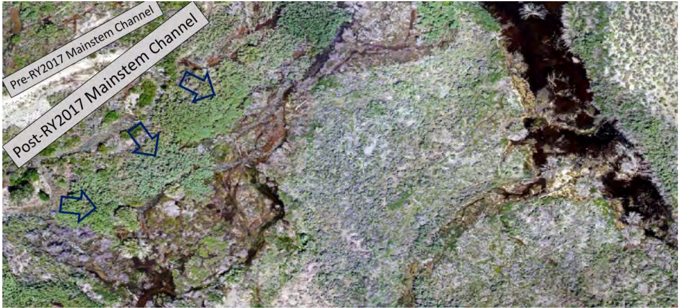
Figure 50. Lower and Central 4-Floodplain with mainstem streamflow access left-to-right. Directional Blue Outlined Arrows for mainstem surface streamflows and late-summer/autumn seepage. CalPoly Humboldt UAV Survey on August 3, 2023. Q_{AV} = 320 cfs.
